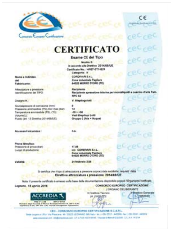
CE certification in accordance with 2014/68/UE Pressure Equipment regulations relevant to pressure vessels
